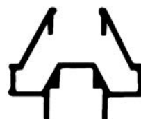
ALG N21 Vidrio perimetral 0.340 kg/m
