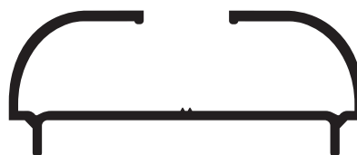
ALG 3103 Contravidrio 12mm 0.447 kg/m
