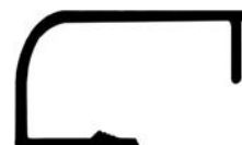
ALG M9 Contravidrio curvo 29mm 0.210 kg/m
